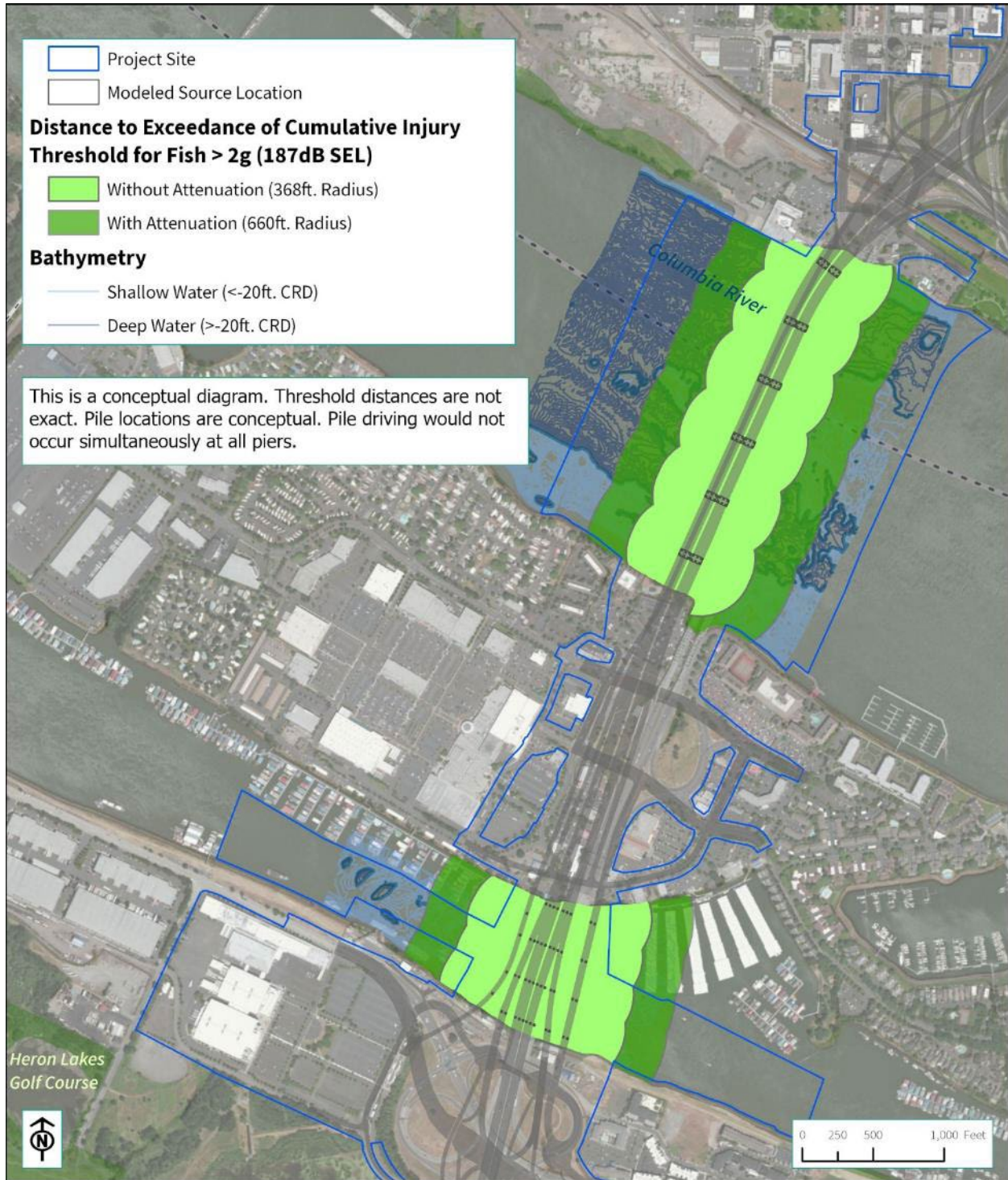
Figure 8-3. Distance to 187 dB SEL Cumulative Injury Threshold for Fish >2 g During Impact Pile Driving – 36 to 48-inch Pile, Single Pile Driver
