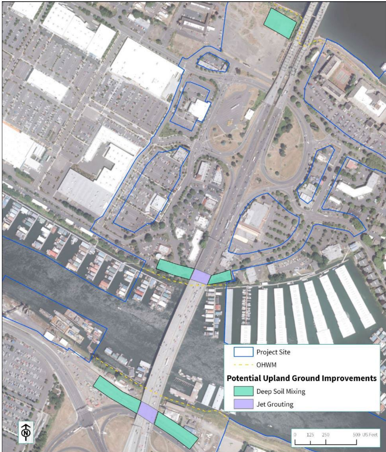
Figure 3-25. Potential Upland Ground Improvements
