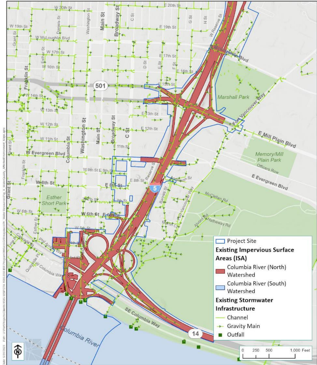
Figure 3-33. Stormwater Existing Conditions – Washington (South)
