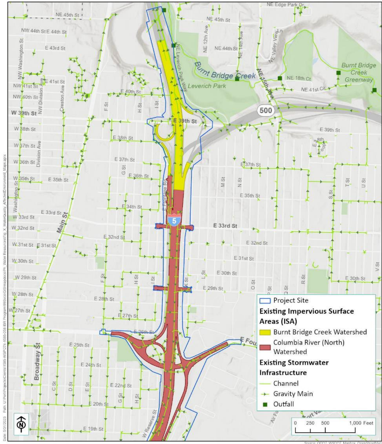
Figure 3-34. Stormwater Existing Conditions – Washington (North)
