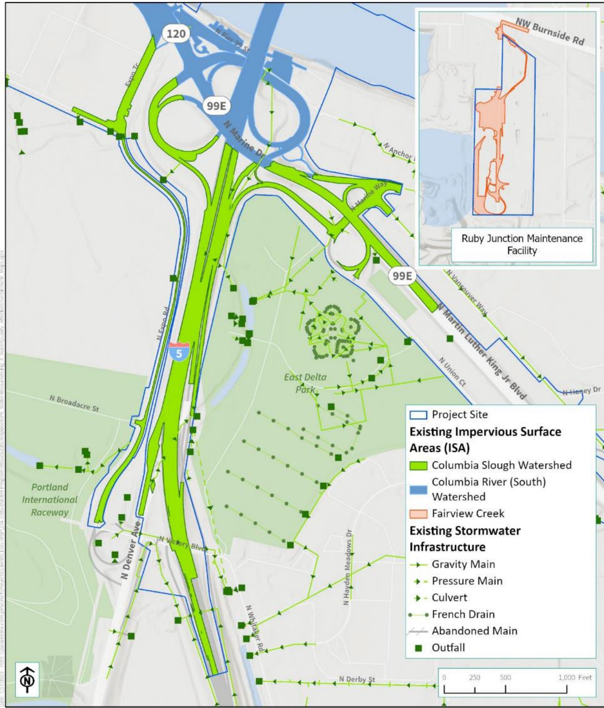
Figure 3-31. Stormwater Existing Conditions – Oregon (South)
