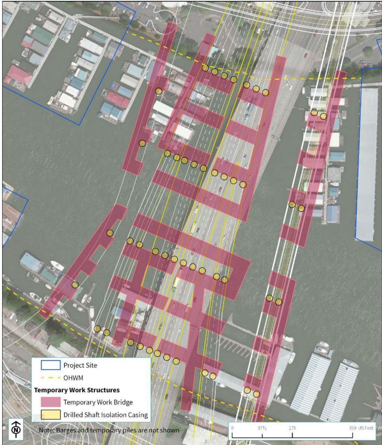
Figure 3-24. Temporary Work Structures – North Portland Harbor
