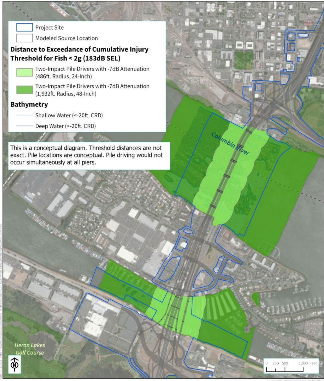
Figure 8-8. Distance to 183 dB SEL Cumulative Injury Threshold for Fish <2 g During Impact Pile Driving – All Pile Sizes, Multiple Pile Drivers
