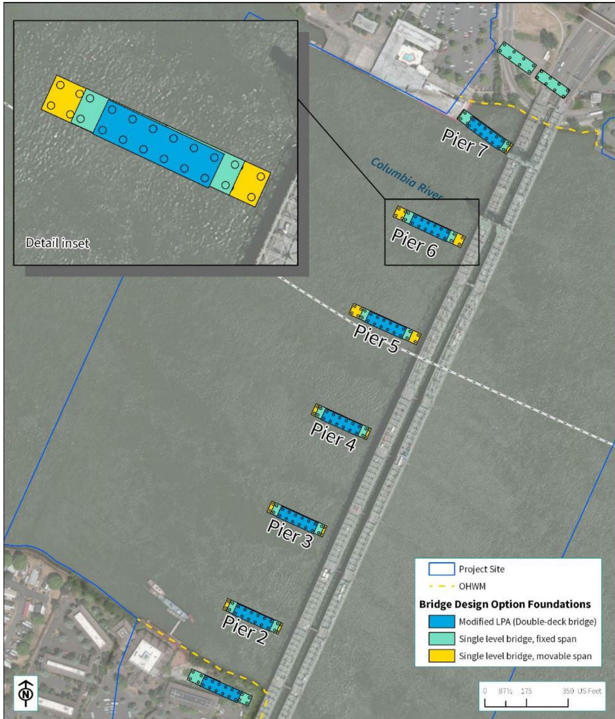
Figure 3-27. Columbia River Bridges – Design Option Foundations
