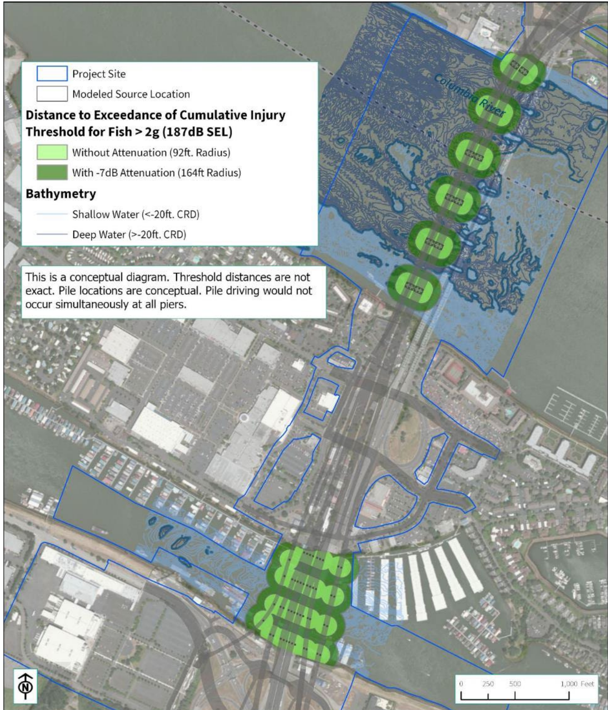
Figure 8-4. Distance to 187 dB SEL Cumulative Injury Threshold for Fish >2 g During Impact Pile Driving – 18 to 24-inch Pile, Single Pile Driver
