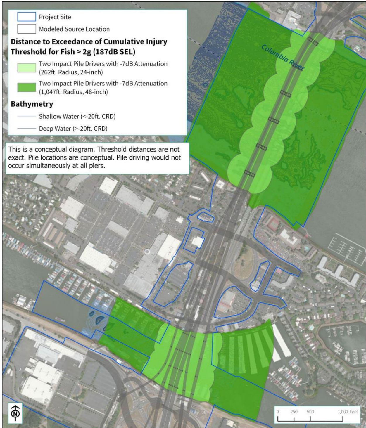
Figure 8-5. Distance to 187 dB SEL Cumulative Injury Threshold for Fish >2 g During Impact Pile Driving – All Pile Sizes, Multiple Pile Drivers
